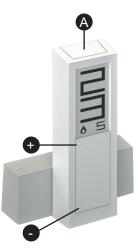
5 Select with the keys "+" or "-" of the hygge programmable thermostat the first free channel (marked by the writing "NEW DEVICE" - for example n°2).
