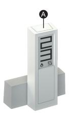
To switch from one display mode to the other, simply hold down the 'A' key (for 8 seconds) until the new display screen appears.
