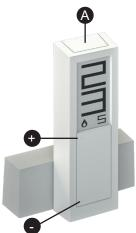
2 Using the "+" and "-" keys, select the device to be deleted from the programmable thermostat memory.
